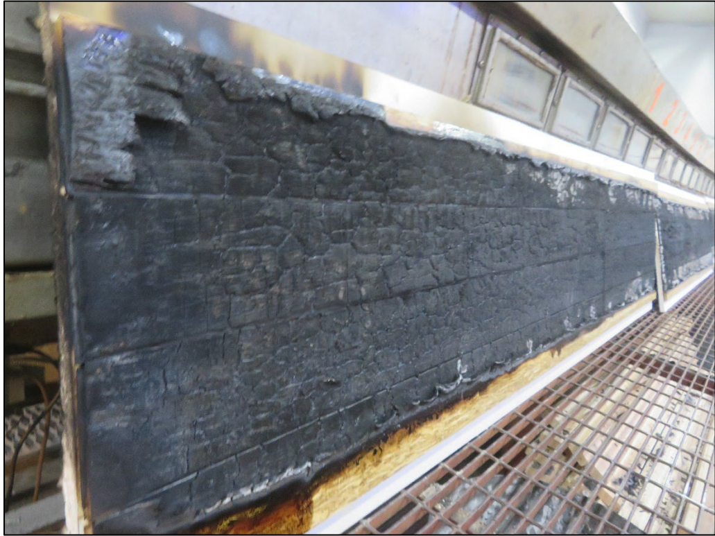
Figure B-3. Exposed Side of the Material After Exposure.
